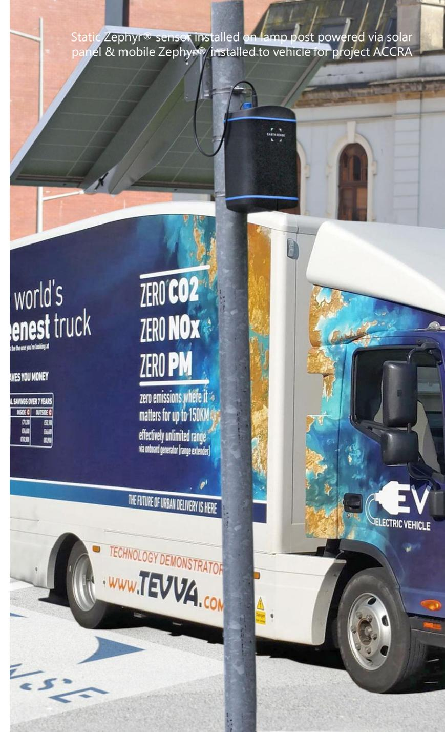
Static Zephyr sensor installed on lamp post powered via solar panel & mobile Zephyr installed to vehicle for project ACCRA
