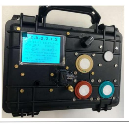
~1.5kg (Include battery) • Weight: <10W (5V, 2.1A, • Power: while recharging) • Battery life: 7.5h
