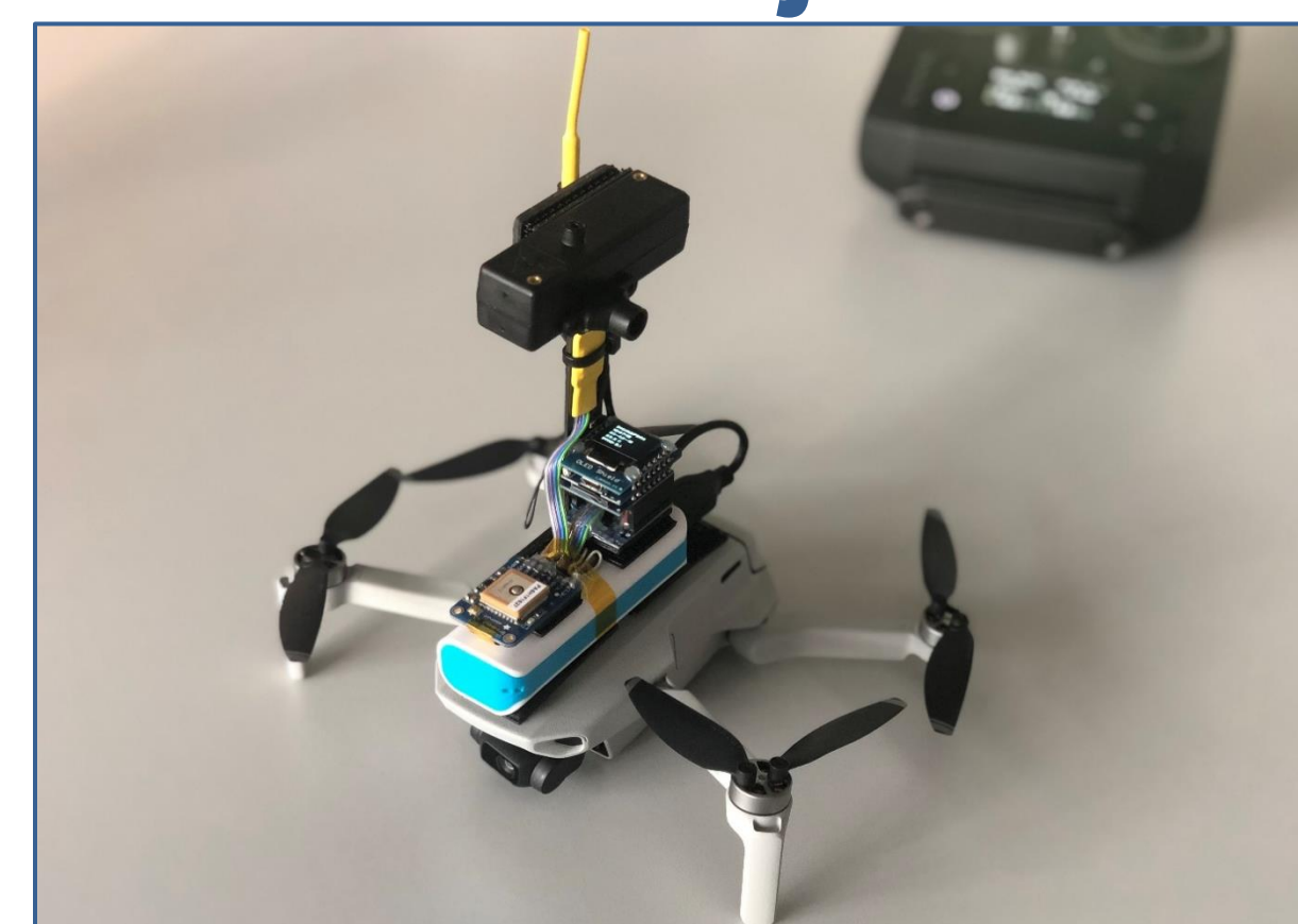
Fig. 6: OPC on tiny drone for industrial indoor-measurements or swarm applications
