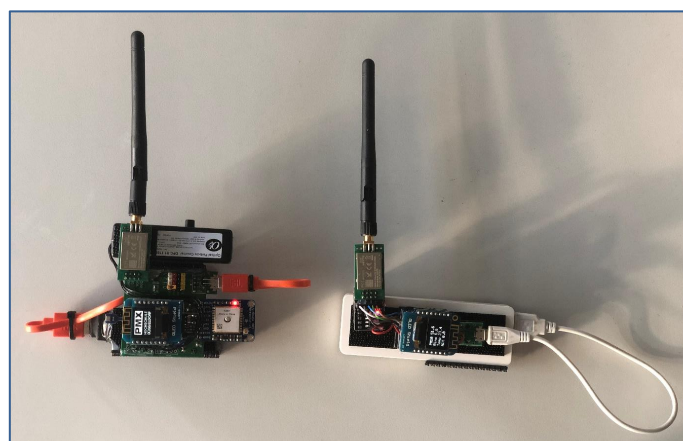
Fig. 7: Measurement data transmission in real time up to 2 km distance
