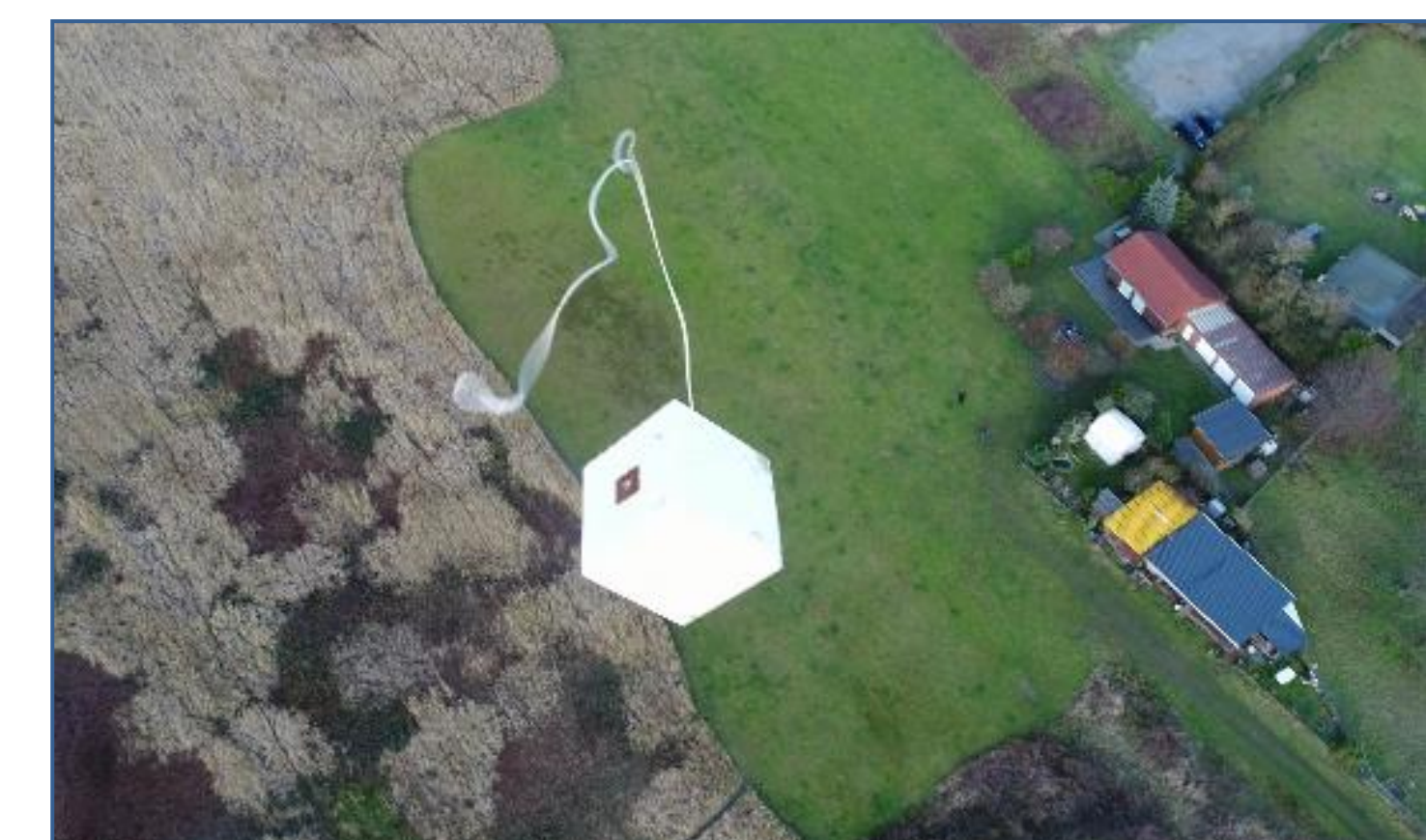
Fig. 9: First functional prototype of the drop-sonde with \text{CO}_2 measurement system and data transmission
