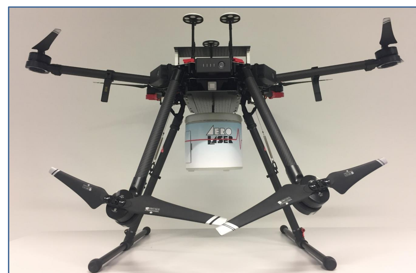
Fig. 8: Development of mobile system capable for industrial and volcanic \text{SO}_2 flux measurements
